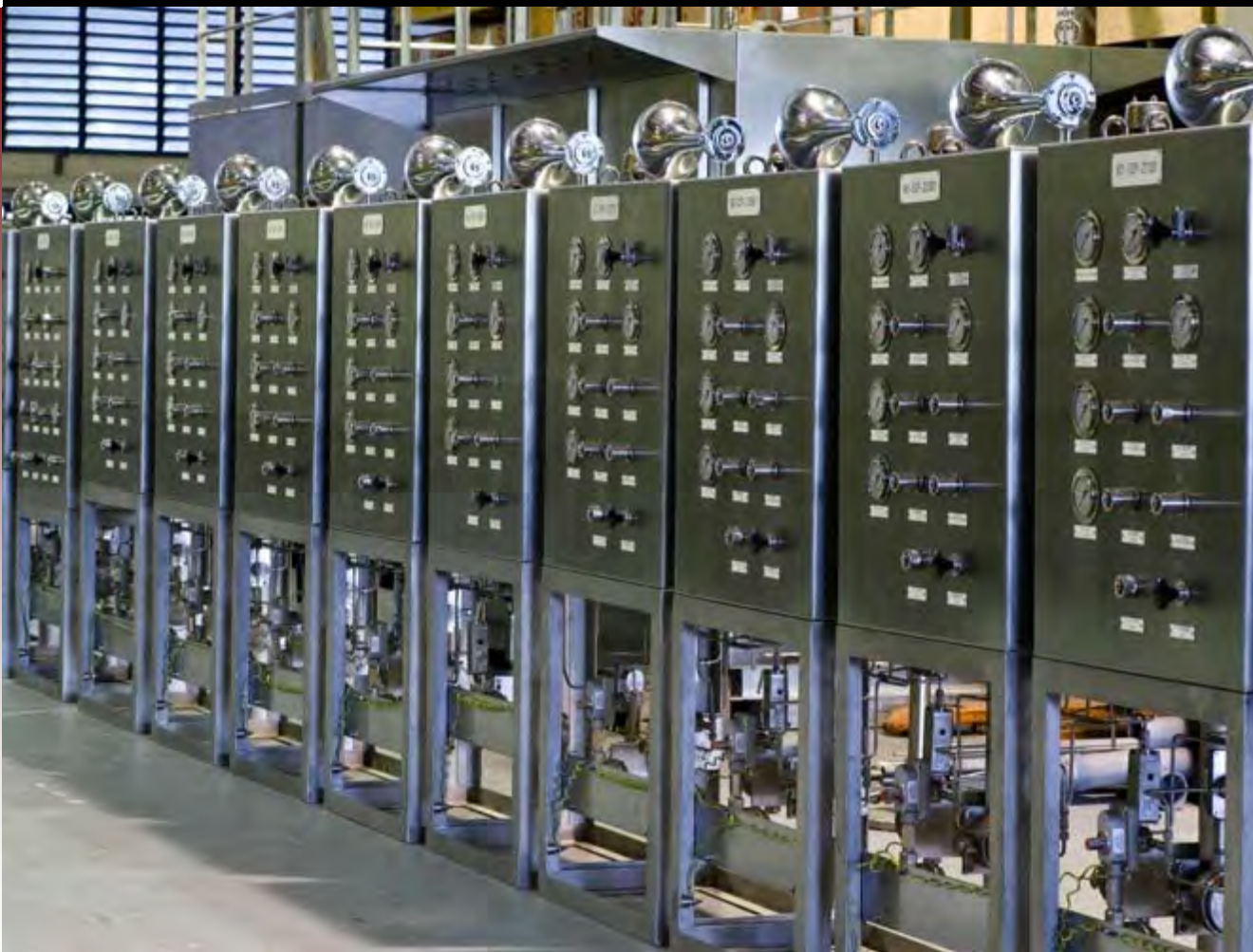
Wellhead control panels INDIA
